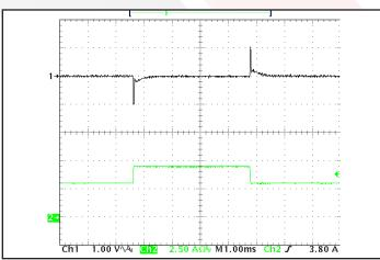
Figure 5: Output voltage response to step-change in load current (50%-75%-50% of lout(max);  $dI/dt = 0.1A/\mu s$ ). Load cap:  $15\mu F$  tantalum cap and  $1\mu F$  ceramic cap. Ch 1: Vout, Ch 2: lout.
