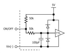
Figure B: Internal ON/OFF pin circuitry
