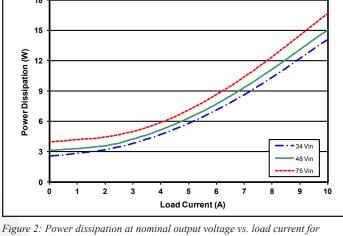
minimum, nominal, and maximum input voltage at 25°C.
